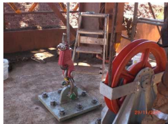
Paraburdoo Train Load-out Conveyor 25 (CV25) – New Hybrid Take-up System. Designed, Procured and Implemented During a Three Days Maintenance Shut Down at Paraburdoo Mine in 2007 in Western Australia.
