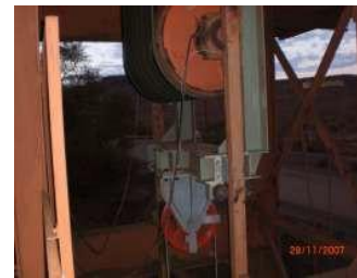
Paraburdoo Train Load-out Conveyor 25 (CV25) – New Hybrid Take-up System. Designed, Procured and Implemented During a Three Days Maintenance Shut Down at Paraburdoo Mine in 2007 in Western Australia.
