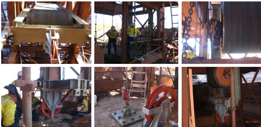
Paraburdoo Train Load-out Conveyor 25 (CV25) – New Hybrid Take-up System. Designed, Procured and Implemented During a Three Days Maintenance Shut Down at Paraburdoo Mine in 2007 in Western Australia.
